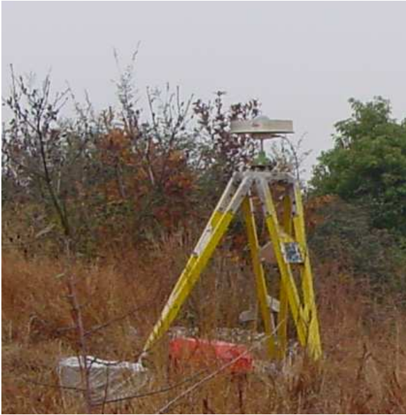
Point 5: heavy tripod for temporary point during GPS observations
