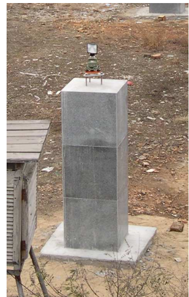
Tribrach and target on DORIS support
