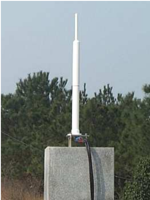
DORIS antenna on its pier
