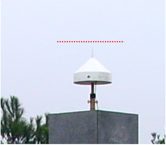
EGNOS station : Novatel antenna on its support
