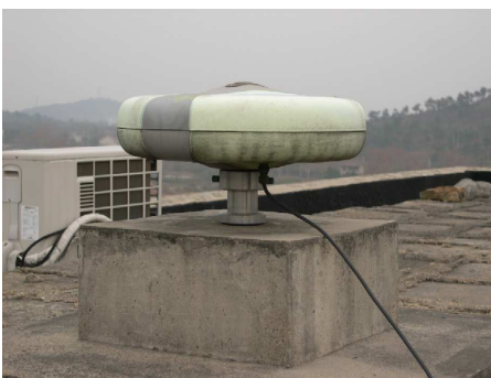
WHJF GPS station antenna
