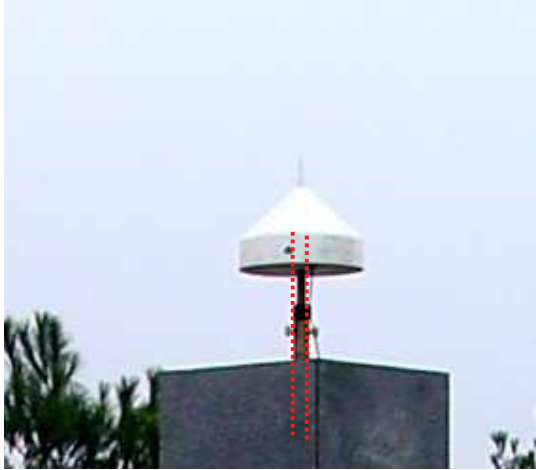
EGNOS station : Novatel antenna on its support
