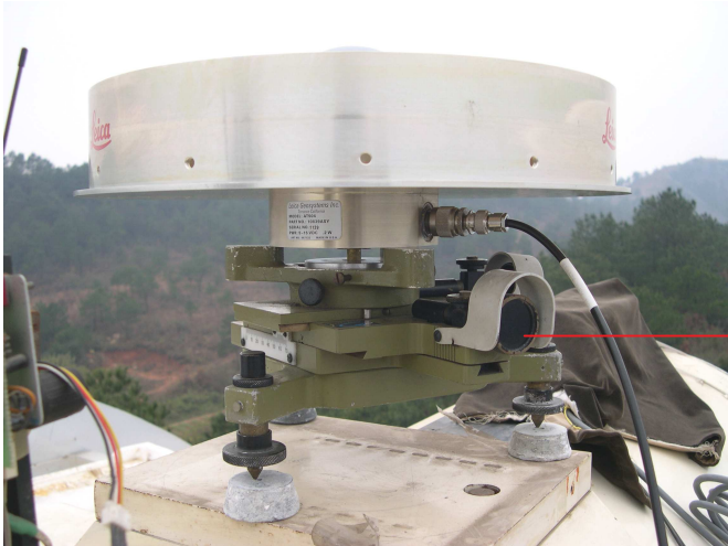
Choke ring antenna set up on the translation stage which is put on top of the SLR and is centered on the SLR vertical rotation axis
