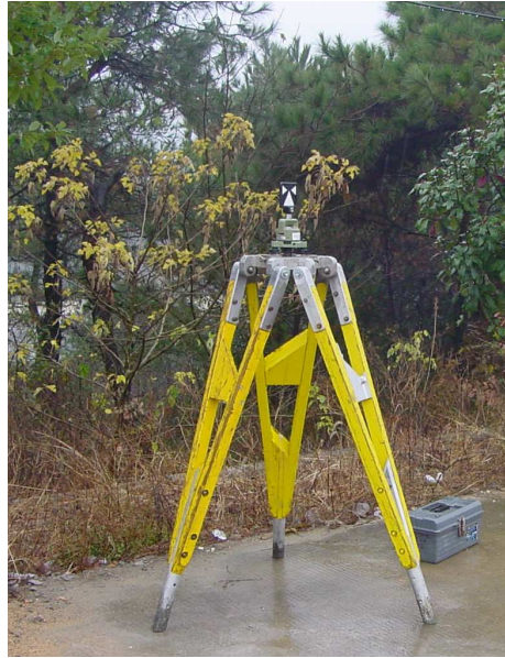
Point 3: Heavy tripod for temporary point during topometric measurements
