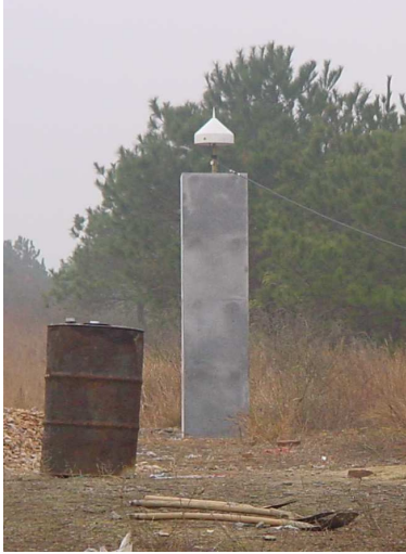
Choke Ring antenna of EGNOS GPS station
