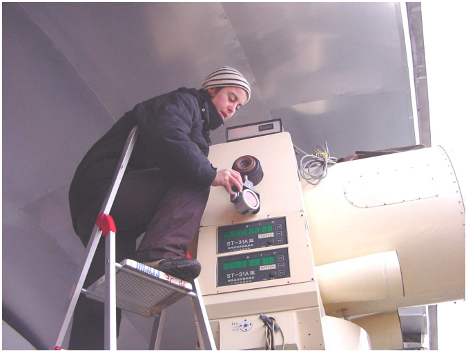
Determination of the vertical eccentricity by indirect levelling
